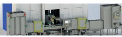
The loading of the parts into the machine is done manually or by automatic system: manipulator, robot, gantry...
