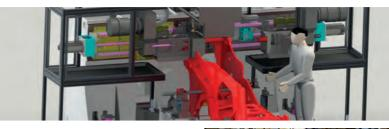
The loading of the parts into the machine is done manually or by automatic system: manipulator, robot, gantry...
